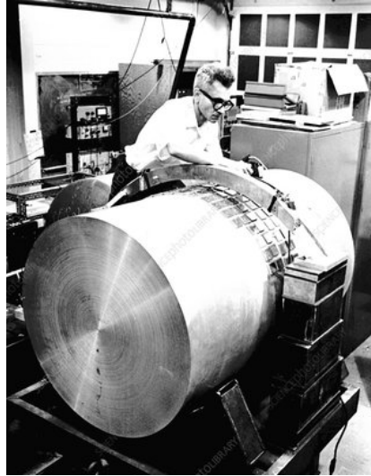
Fig. 2. Joseph Weber with his resonant mass detector 4
